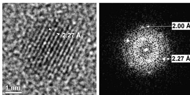
**Fig. 5** (Left) HRTEM image showing the fringes of the palladium nanoparticles (sample B). (Right) Fast Fourier transform revealing the lattice periodicities of the palladium nanoparticles.
