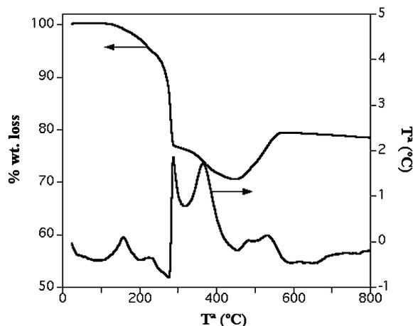
**Fig. 6** TGA (above) and DTA (below) data for the solid sample A palladium nanoparticles.
