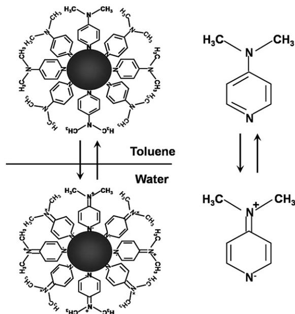
**Fig. 2** Scheme of the experimental procedure used to transfer the Pd nanoparticles prepared in toluene into the aqueous phase. The phase transfer agent, dimethylaminopyridine (DMAP), neutral in the organic phase, is able to quantitatively extract the nanoparticles into the aqueous phase, where it is present as its zwitterion tautomeric form.
