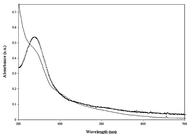
**Fig. 3** Optical absorption spectra of an aqueous  $[\text{PdCl}_4]^{2-}$  solution (dotted line) and a suspension of Pd/TOAB nanoparticles in toluene (solid line).
