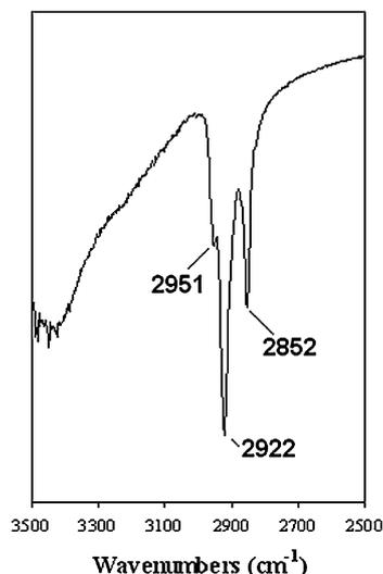
**Fig. 4** KBr diluted FT-IR spectrum of solid palladium nanoparticles capped with TOAB (sample A).
