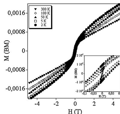
**Fig. 8** Magnetisation hysteresis loops for Pd nanoparticles (sample B) at 2, 5, 50, 100, and 300 K.
