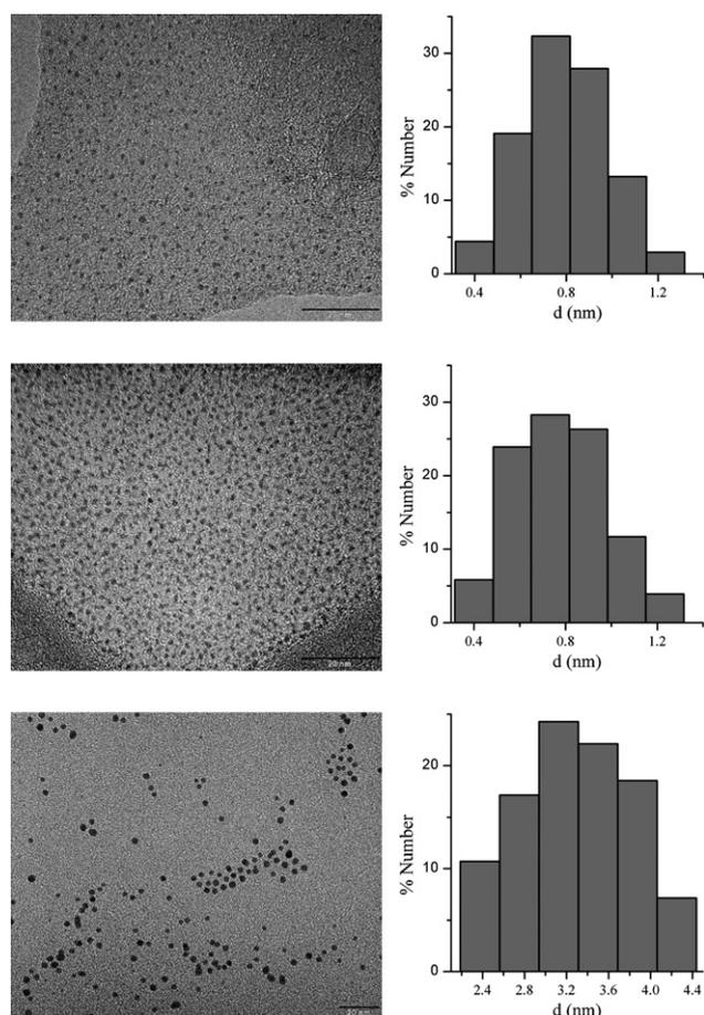
**Fig. 1** Transmission electron micrograph of sub-nanometer (sample A) and 3.5 nanometer (sample B) palladium particles (top and bottom respectively) prepared by reduction of  $[\text{PdCl}_4]^{2-}$  with  $\text{NaBH}_4$  in toluene. (Middle) Sample A nanoparticles after transfer into the aqueous phase. The scale bar represents 20 nm.
