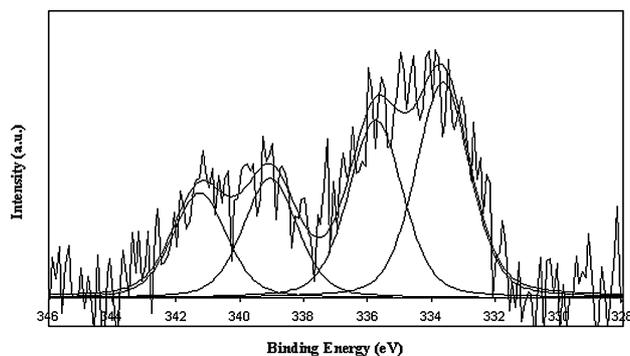
**Fig. 7** XPS spectrum of a solid sample A of TOA-capped Pd nanoparticles.
