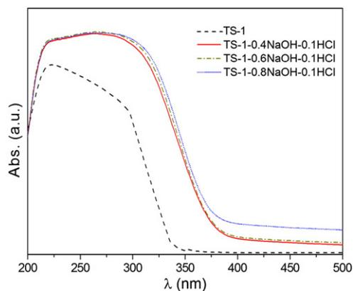
Fig. 4. UV-vis spectra of parent TS-1 and desilicated TS-1 zeolites.
