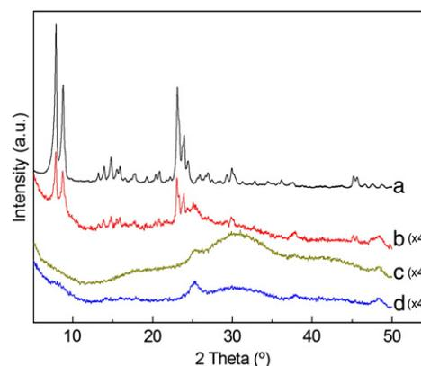
**Fig. 2.** XRD patterns corresponding to the (a) original TS-1 zeolite and TS-1 treated with NaOH (b) 0.4 M, (c) 0.6 M and (d) 0.8 M, followed by a 0.1 M HCl washing step. Spectra have been vertically shifted for clarity.
