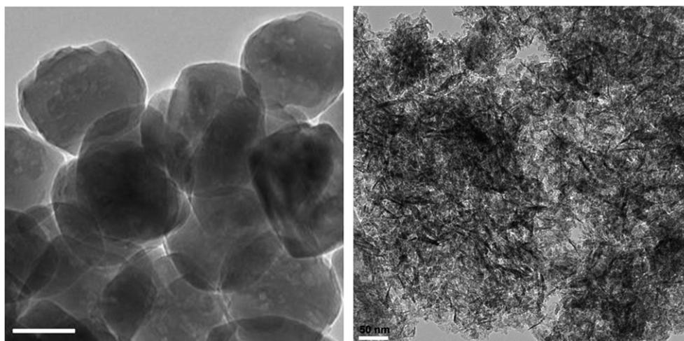
**Fig. 1.** Representative TEM micrographs of the original TS-1 zeolite (left, scale bar = 100 nm) and TS-1 desilicated samples using NaOH 0.4 M followed by the HCl solution post-synthetic treatment (right, scale bar = 50 nm).
