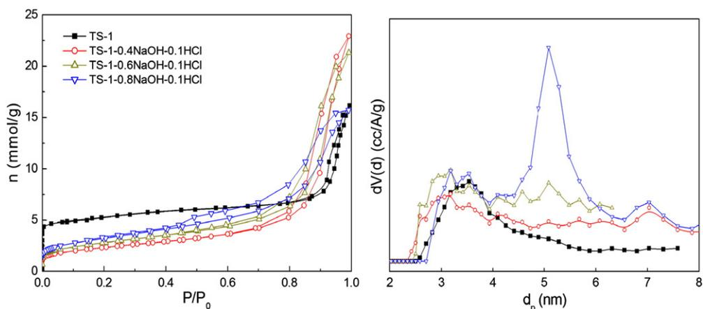
Fig. 3.  $N_2$  adsorption–desorption isotherms (left) and the corresponding pore size distributions calculated by applying NL-DTF to the absorption branch (right) for the parent TS-1 and the desilicated samples.
