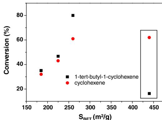
Fig. 5. Correlation between catalytic activity and BET surface area for the different desilicated TS-1 samples for the oxidation of cyclohexene and 1-*tert*-butyl-cyclohexene.
