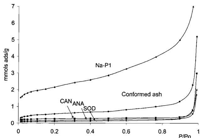
Figure 7. Isotherms of N<sub>2</sub> at 77 K of the conformed ashes, Na-P1, cancrinite, analcime and sodalite.
