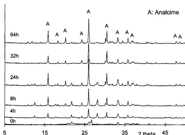
**Figure 4.** Evolution of the conformed ashes treated in 1 mol dm<sup>-3</sup> NaOH at 431 K for different periods of time, analysed by XRD.
