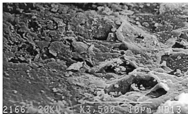
Figure 3. SEM image of the conformed ashes.
