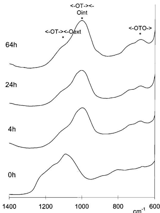
**Figure 5.** Evolution of the conformed ashes treated in 1 mol dm<sup>-3</sup> NaOH at 431 K for different periods of time, analysed by DRFTIR.
