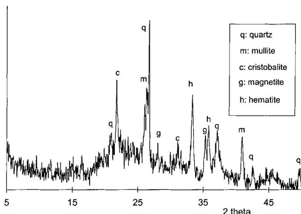
Figure 2. XRD pattern of the conformed ashes used as raw material.
