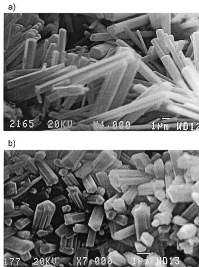
Figure 8. SEM images of some zeolites prepared by hydrothermal treatment; (a) zeolite Na-P1 and (b) cancrinite.
