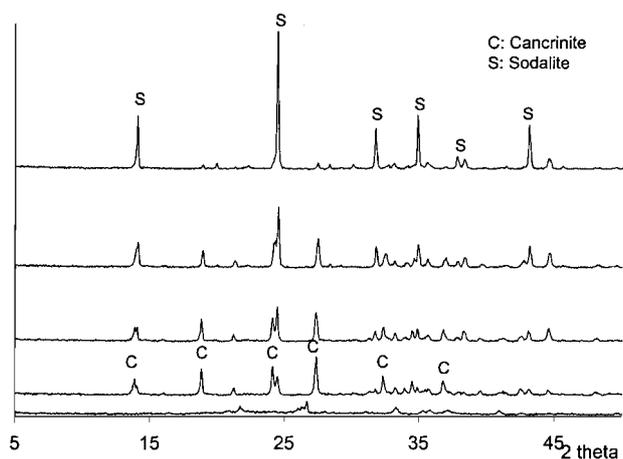
Figure 6. Evolution of the conformed ashes treated in 10 mol dm<sup>-3</sup> NaOH at 463 K for different periods of time, analysed by XRD.
