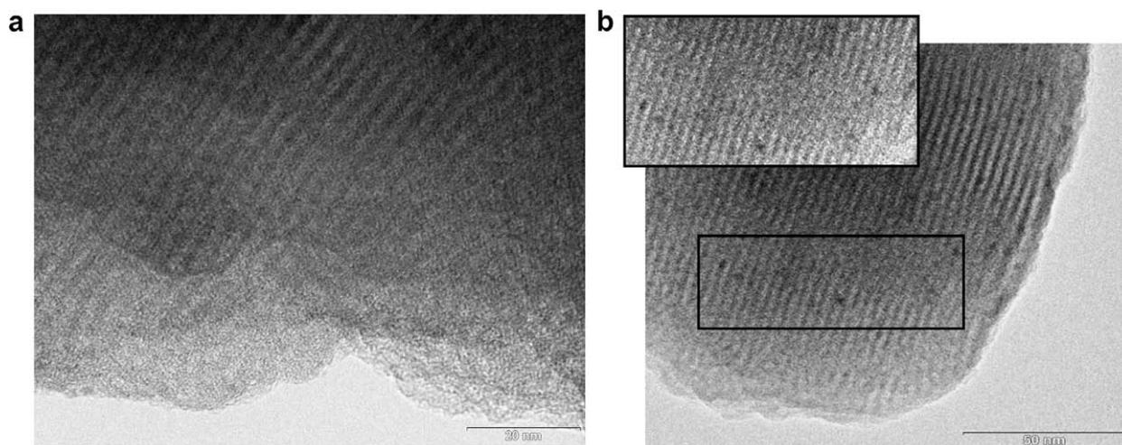
**Fig. 8.** Representative TEM micrographs of Pd nanoparticles incorporated in MCM-41 using triethoxysilane-functionalized Pd nanoparticles (a) before and (b) after calcinations. The scale bars represent 20 and 50 nm, respectively.
