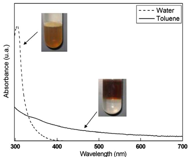
**Fig. 3.** Optical absorption spectra of Pd/tetraoctylammonium nanoparticles in toluene (continuous line) and aqueous Pd/DMAP nanoparticles (dotted line). The insets display the corresponding test tubes containing Pd nanoparticles before and after phase transfer.
