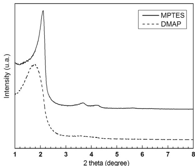
Fig. 6. X-ray diffraction patterns of a sample prepared by hydrolysis of TEOS in the presence of CTAB and triethoxysilane-functionalized Pd nanoparticles (top) and DMAP-functionalized Pd nanoparticles (bottom).
