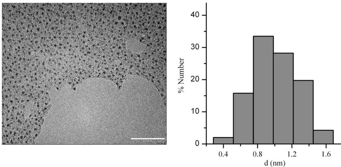
**Fig. 1.** Transmission electron microscopy (TEM) micrograph of Pd nanoparticles prepared by reduction of  $[\text{PdCl}_4]^{2-}$  with  $\text{NaBH}_4$  in toluene while stirring at 1600 rpm. The scale bar represents 20 nm.
