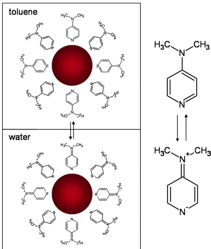
**Fig. 2.** Scheme of the experimental procedure used to transfer the Pd nanoparticles prepared in toluene to the aqueous phase. The transfer agent, dimethylaminopyridine (DMAP), neutral in the organic phase, is able to quantitatively extract the nanoparticles to the aqueous phase, where it is present as its zwitterion form. Adapted from Ref. [45].
