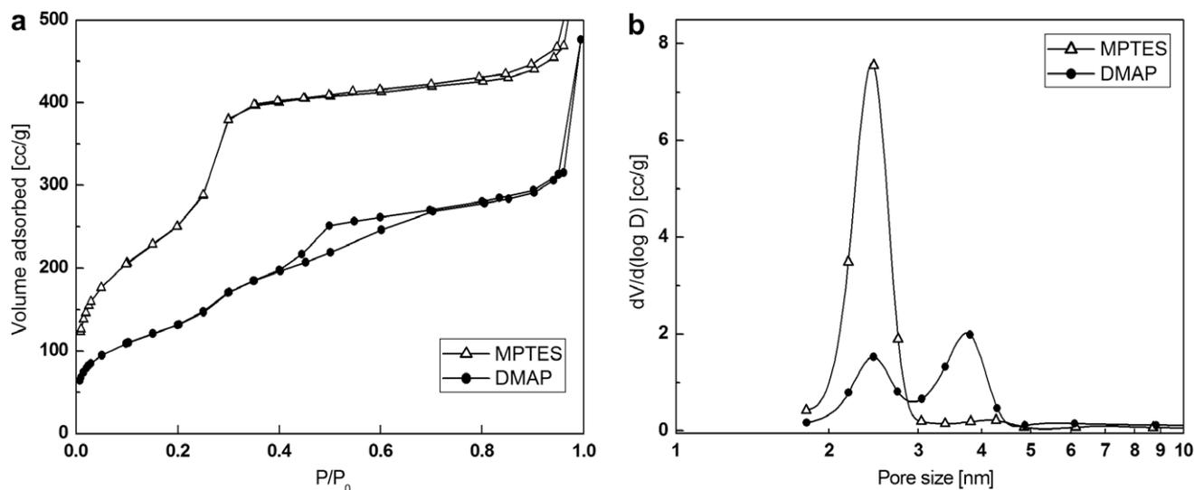
**Fig. 7.** (a) Nitrogen adsorption/desorption isotherms at 77 K and (b) corresponding pore size distribution (BJH method) of a sample prepared by hydrolysis of TEOS in the presence of CTAB and triethoxysilane-functionalized Pd nanoparticles (top, triangles) or DMAP-functionalized Pd nanoparticles (bottom, circles).
